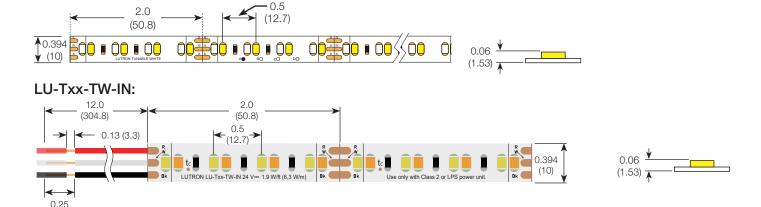
CAUTION: Overheating Risk. May result in moderate injury or product damage. Do not power the LED tape while coiled, on a spool, or directly to 120 V~ power/line voltage. Unroll or install before applying power.
