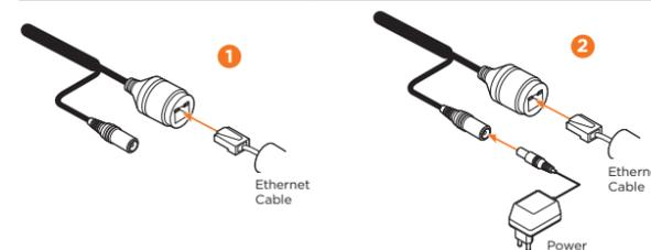
STEP 3 - INSTALLING THE CAMERA
