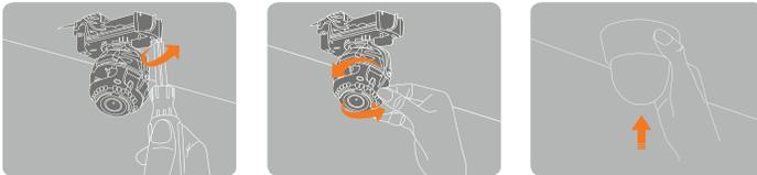
1 Two Screw Installation      2 Adjustment      3 Snap It
