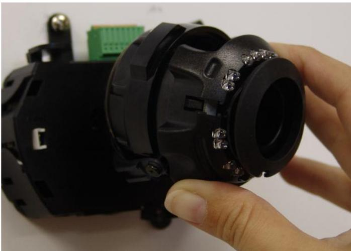
3. Adjust the camera's position using the 3-Axis Gimbal.
