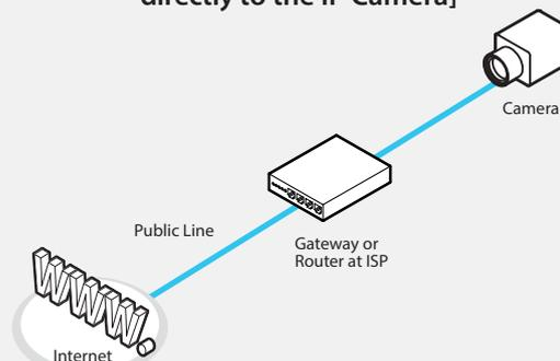
**i** To connect the IP camera directly to a modem, power down and reset the modem. Leave the modem powered down until configurations are finalized with the IP camera and the IP camera has been connected correctly to the modem. Then power on the modem, followed by the IP camera.
