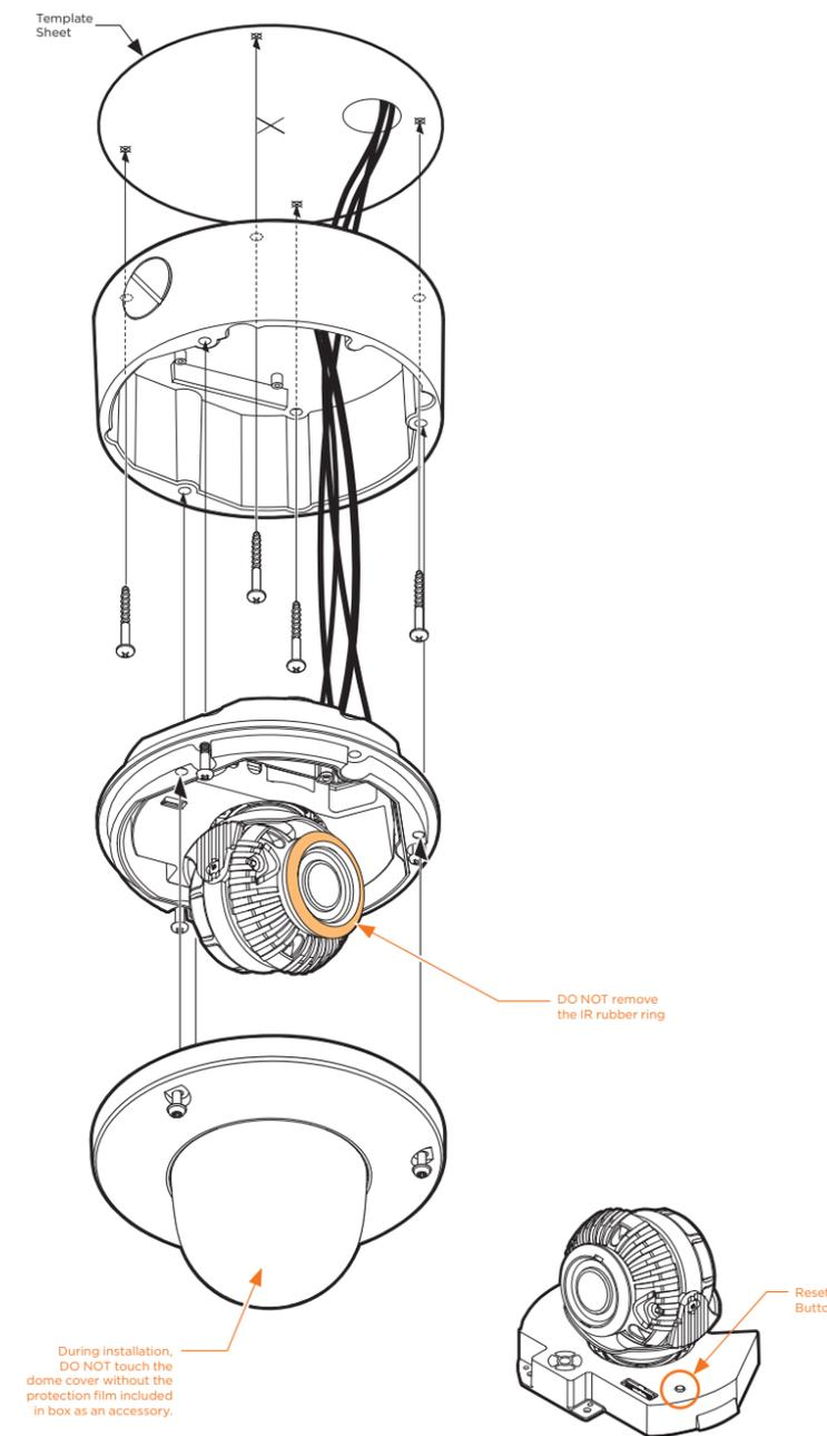
During installation, DO NOT touch the dome cover without the protection film included in box as an accessory.
