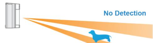
No alarm when only the lower detection area is triggered.
