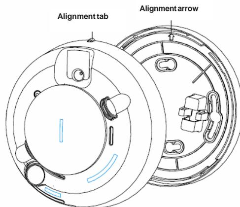
Note: The product is designed so that it cannot be attached to the mounting base if no batteries are installed.
