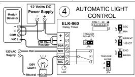
For turning on an interior or exterior light with a motion detector. When motion is detected, the ELK-960 is triggered and the light is turned on. The amount of time the light remains on after the detector resets is adjustable. Delay time will automatically restart each time the motion detector activates.
