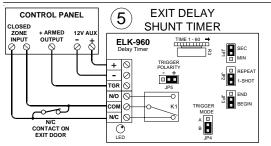
Provides an exit delay to an otherwise instant alarm loop.
