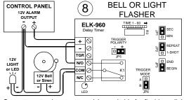
Converts a steady output to pulsing, suitable for flashing a light or pulsing an audible device. Note: Alarm output must be capable of supplying enough current to drive the bell and light.
