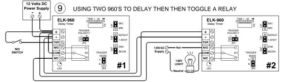
Used for delaying a trigger then toggling a relay on/off. ELK-960 #1 starts a time delay when the N/O switch is closed. When 960 #1's time delay expires, 960 #2 is triggered turning it's relay on for the time delay setting, then turning the relay off. (toggle) To sumarize: fire trigger on #1, waits, turns on #2's relay, waits, then turns relay off.
