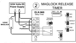
Used to extend the release time of an access control device or to manually activate a door **maglock** release device. The trigger is activated by a contact closure or a N/O pushbutton and the door maglock remains released (door open) after the button is released for the delay time set up in the ELK-960.
