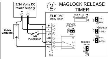
Used to extend the release time of an access control device or to manually activate a door **maglock** release device. The trigger is activated by a contact closure or a N/O pushbutton and the door maglock remains released (door open) after the button is released for the delay time set up in the ELK-960.
