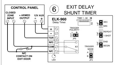
Provides an exit delay to an otherwise instant alarm loop. The ELK-960 is triggered by the control's Armed output. The door contact is then shunted by the relay contacts. After the user has exited and the delay time has expired, the door contact is restored into the loop.
