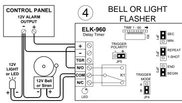
Converts a steady output to pulsing, suitable for flashing a light or pulsing an audible device. Note: Alarm output must be capable of supplying enough current to drive the bell and light.
