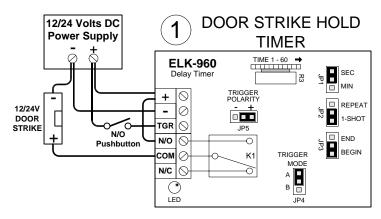
Used to extend the release time of an access control device or to manually activate a door **strike** release device. The trigger is activated by a contact closure or a N/O pushbutton and the door strike remains activated (door open) after the button is released for the delay time set up in the ELK-960.
