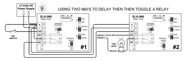
Used for delaying a trigger then toggling a relay on/off. ELK-960 #1 starts a time delay when the N/O switch is closed. When 960 #1's time delay expires, 960 #2 is triggered turning it's relay on for the time delay setting, then turning the relay off. (toggle) To sumarize: fire trigger on #1, waits, turns on #2's relay, waits, then turns relay off.
