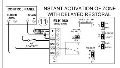
When contact opens, relay is turned on which causes instant zone violation. Contact reclosure will cancel trigger applied by resistor. Delay starts when contact closes. Relay turns off and zone restores after delay time expires.
