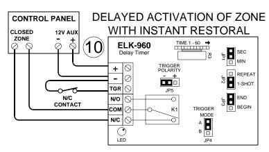
Contact closure applies a constant trigger which keeps relay off and zone closed. Delay starts when contact opens. After delay time expires, the relay turns on and the zone is activated (opened). Closing the contact restores the zone instantly.
