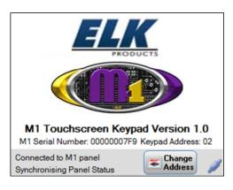
The Start-up screen displays until all current status data is collected from the M1 panel. Once this is complete the keypad will move on to the following MAIN USER screen.
