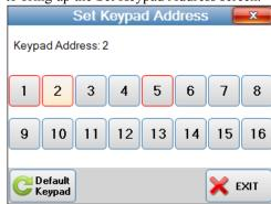
NOTE: If the Main User Screen is displayed then pressing and holding the "CLEAR" key for 15 seconds will bring up the Set Keypad Address screen.
