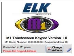
It an address is not set it will display "Please Set Keypad Address". If "Waiting to connect to panel" is displayed then a data bus enrollment needs to be performed from an already enrolled keypad.
