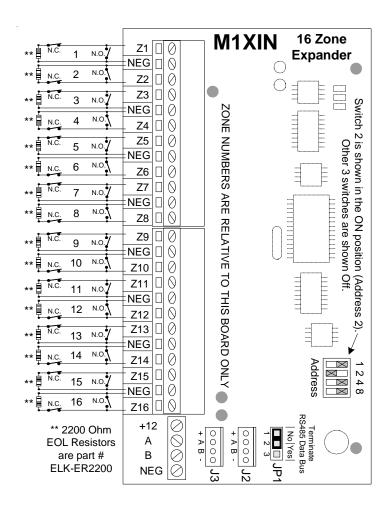
The Data Bus Address is set by the group of 4 miniature slide switches. Starting from the end, each switch has a position of 0 or 1 (OFF/ON) and a decimal equivalent of (1, 2, 4, or 8). The total decimal value of the switches turned "ON" equals the address setting. The address setting in turn defines which input zones (in banks of 16) are assigned to the expander. Inputs Expanders are factory set to address setting 2 (Zones "Inputs" 17 to 32).
