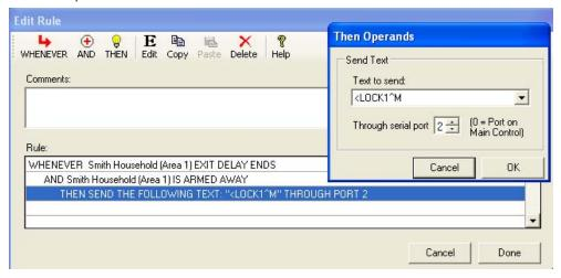
6.15 Be sure that ElkRP is connected and on-line with the M1 Control, then click Send to Control.
