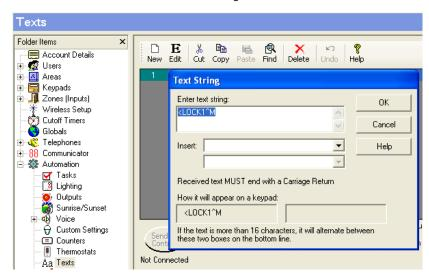
Example: Text String "**<LOCK1^M**" is the command to lock the first Z-Wave Lock (LOCK1). See Table 6 for additional Text Strings that may be sent to control locks.
