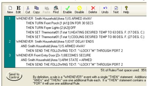
Rule 1 - When the System is Armed to Away mode this rule will turn on the Flood lights for 30 sec., turn off the Foyer Lights, and change the HVAC Thermostat Settings. This is typical of an Energy Save type of rule.
