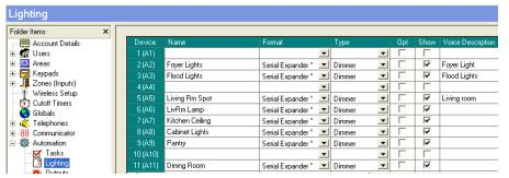
NOTE: All Z-Wave devices are assigned Node IDs, but ONLY those that are lighting types should be entered in the M1 Light Device locations. Leave empty (blank) any location that corresponds to a Node ID that is NOT a light device.
