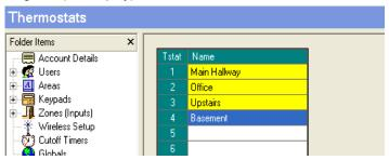
**TIP!** If the customer wants the Thermostats to appear in a desired order then it will be necessary to perform the Z-Wave Inclusion in exactly that desired order. That's because the order of mapping in M1 is based solely on the Z-Wave Node ID numbering starting at the lowest and working up. Remember that M1 rules reference the Thermostat Name, making it VERY important for each name to describe and/or match the correct location.
