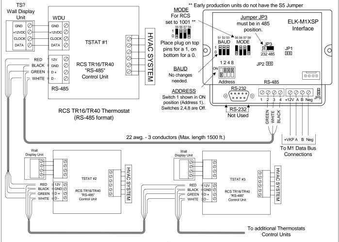
Thermostat brand, interface format, and model of ELK-M1 Control dictates the total number of thermostats allowed. The M1G supports up to 16 of the RCS-TR16/TR40 (RS-485 models) using a single (1) M1XSP.
