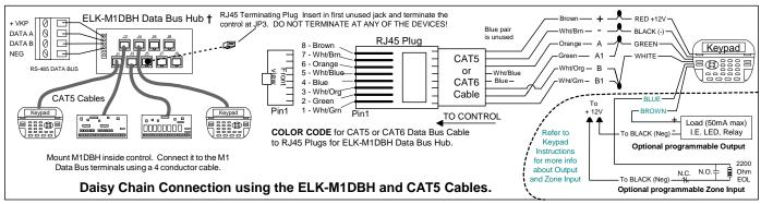
The optional ELK-M1DBH † Data Bus Hub is suggested if the job must have more than 2 home runs. The M1DBH accepts CAT5 or CAT6 cable with RJ45 plugs. It keeps wires more organized while also providing easy bus termination. Essentially, the M1DBH circuit board daisy chains the devices by series connecting the DATA lines A & B. An plug-in RJ45 terminator is supplied for use in the first unused jack.
