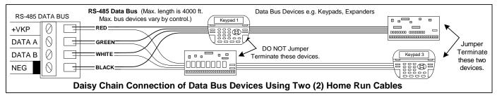
The M1 should have no more than 2 home run cables but devices can be daisy chained along each. The last device on each home run SHOULD be terminated via the gold 2 pin terminating header/jumper. Placing a shorting cap on the pins will engage a 120 Ohm resistor across data lines A & B. If there is only 1 data bus home run cable then place shorting cap on JP3 of Main Board. See other hookups below.
