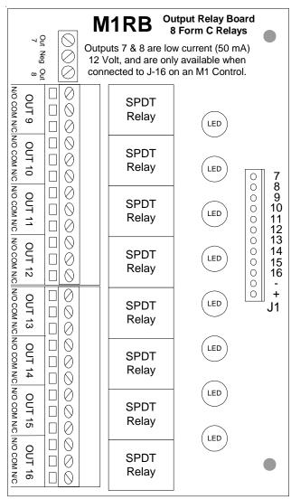
The relay output numbers are relative ONLY when connected to J-16 on an M1 Control. If connected to an Output Expander, the numbers must be mapped to the appropriate numbers of the expander.
