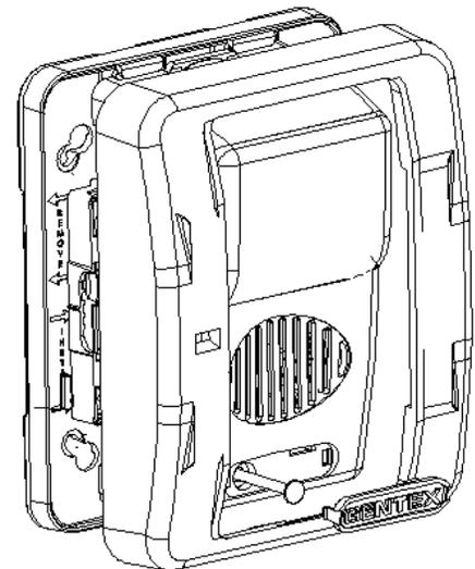
To remove bezel, grip both sides of bezel and pull in a downward and outward motion.
