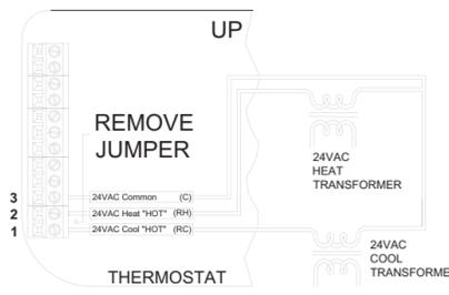
For HVAC systems with separate heating and cooling transformers, the metal jumper between Terminal 1 (RC) and Terminal 2 (RH) on the left terminal strip must be removed.
