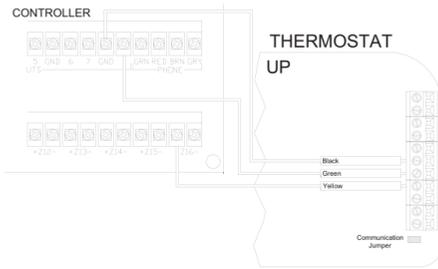
Figure 12 – Connections to HAI Home Control System
