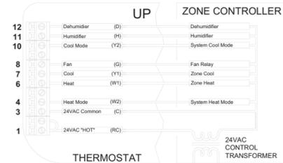
Figure 7 – Connections for single stage thermostat for zone control systems
