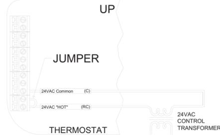
For HVAC systems with a single transformer, the metal jumper between Terminal 1 (RC) and Terminal 2 (RH) on the left terminal strip must remain in place.
