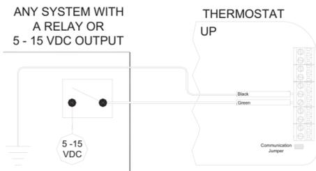
Figure 13 – Connections to a Remote Setback Switch
