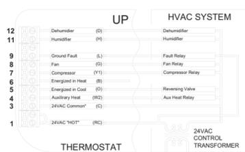
Figure 9 – Connections for heat pump thermostat
