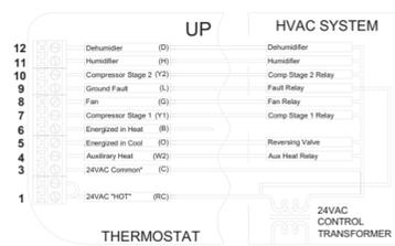
Figure 10 – Connections for two speed heat pump thermostat
