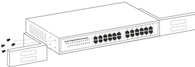
Attach the mounting brackets on the switch's side panels (one on each side) and secure them with the screws provided.
