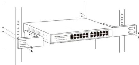
Use the screws provided with the equipment rack to mount the Intellinet data switch on the rack.
