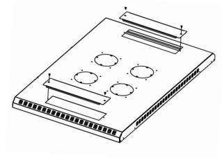
Insert cover into the opening and secure with a screw on either side
