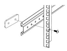
Unscrew the rail from the rail support. Move the rail forwards or backwards to desired location. Insert screw and secure.
