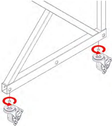
Step 2: Thread each caster all the way in to the insert so that no threads are exposed.
