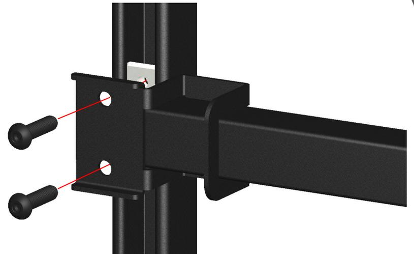
Place Channel Nuts behind inside Flanges of Uprights. Install Bolts through Mounting Bracket into Channel Nuts.
