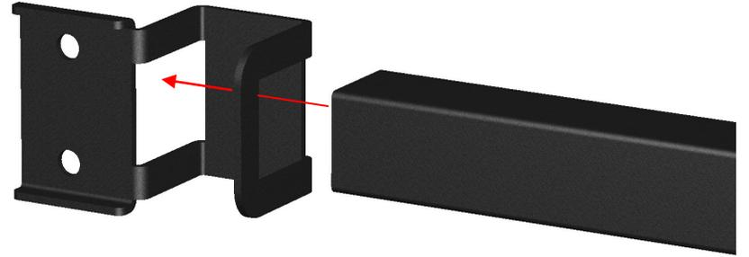
Slide both Mounting Brackets on both ends of Accessory Bar.
