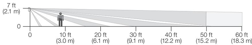
\* Sensor mounting shown at 7 ft (2.1 m). Mounting height should be between 6 ft and 8 ft (1.6 m and 2.4 m).
