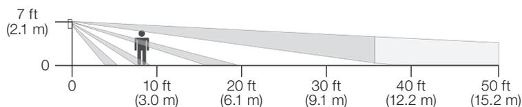
\* Sensor mounting shown at 7 ft (2.1 m). Mounting height should be between 6 ft and 8 ft (1.6 m and 2.4 m).
