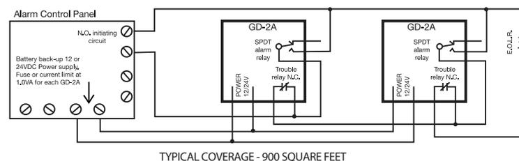
5. The GD-2A uses a full wave bridge rectifier at its power input, so that it is independent of the polarity of the input power. It can operate on DC or AC voltages between 12 and 24 volts.
