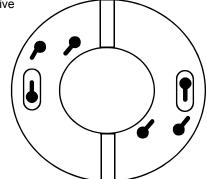
**Step 5. Reinstall the GEM HEAT into the mounting plate.** Align the mounting screws with the mounting holes in the base. Push down and turn clockwise until the GEM-HEAT snaps into place.
