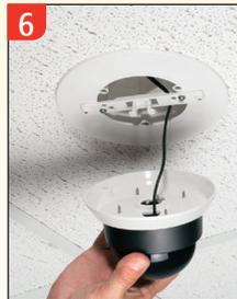
6 With camera mounted, install the mounting plate to the box by placing it on the bracket and turning clockwise to lock. Install set screw.
