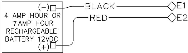
The RED (+) and BLACK (-) flying leads must be connected to a 12VDC 4-7 AH Rechargeable Battery, to serve as backup power in the event of AC Power Failure. **NOTE:** To calculate the available standby time refer to the Standby-Battery Calculation Worksheet at the back of this manual.
