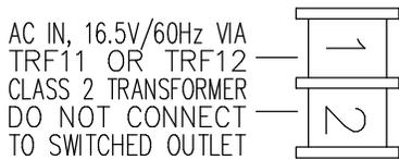
(The following applies to installations in the United States of America): Connect a 16.5 VAC Transformer to Terminals 1 and 2, using a wire of #18 AWG. or larger at a distance of 15 ft. or less from the control panel. **NOTE:** Do not connect to a switched outlet.
