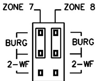
The GEM-P816 can use conventional 12 VDC 4-wire smoke detectors. To use them, select fire zone programming option and do not select 2-wire smoke detector programming option for the desired fire zone (refer to the GEM-P816 Programming Instructions). Set JP3 to the position as shown, if zones 7 or 8 are to be used.
