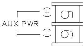
Connect the auxiliary devices (motion detectors, glass breaks, etc.) to Terminals 5 and 6. Auxiliary Power provides 11.7-12.5 VDC nominal output which is used for powering auxiliary devices. **NOTE:** To calculate the available standby time refer to the Standby-Battery Calculation Worksheet at the back of this manual.
