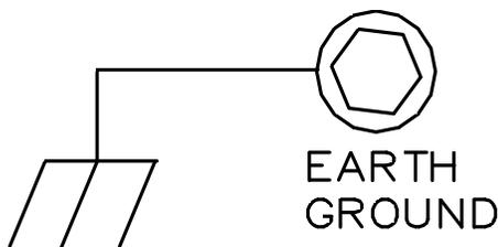
Connect the control panel EARTH GROUND screw to a metal cold-water pipe using at least a #16 AWG. wire. Do not use a gas pipe, plastic pipe or AC ground connections. Also, connect the circuit board to the metal enclosure. Connect a wire with a ground lug crimped or soldered onto one end of the EARTH GROUND screw to the cabinet. **NOTE:** Grounding connections should avoid bends in the grounding wire whenever possible.
