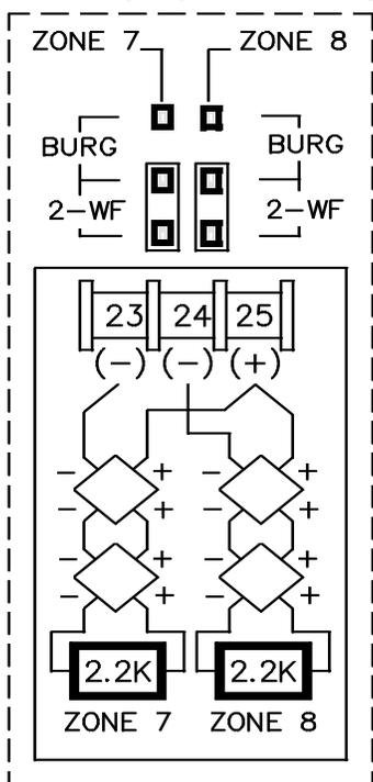
Two-wire smoke detectors can only be connected to zones 7 and 8. To use them, select fire zone programming option and select 2-wire smoke detector programming option for the desired fire zone 7 or 8 (refer to the GEM-P816 Programming Instructions) and set JP3 to the "2-WF" position as shown. Connect the 2-wire smoke detectors as shown.
