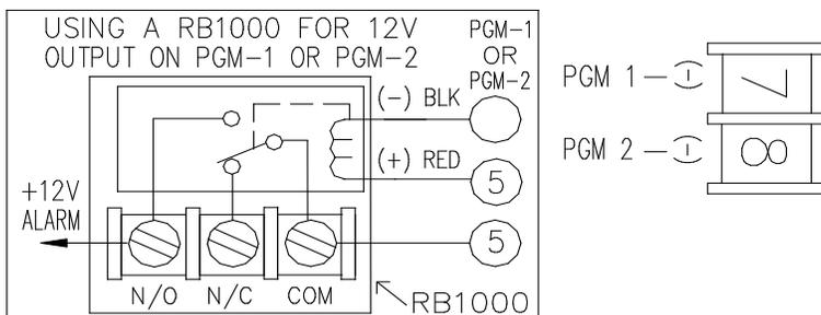
PGM1 and PGM2 are negative switched programmable outputs that can be activated depending on the programming options selected (see GEM-P816 Programming Instructions). Connect the device controlled by the programmable output between terminal 5 (+) and the PGM output (-), either terminal 7 or 8. As an example, the connection to the RB1000 Relay Module is shown.
