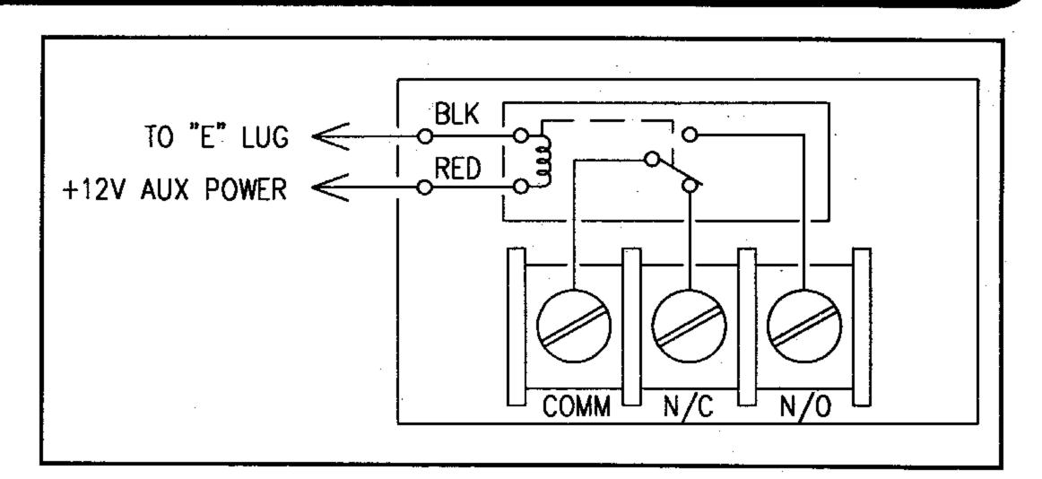
**Note:** (1) For MA1000e: Cut off the spade-lug connector from the BLACK wire and insert the stripped end into Terminal 11. Connect the RED wire to AUX. POWER, Terminal 6. (2) For MA1016e: When using the Voltage Output on Alarm feature (using the Fire Zone as an output), connect the RED wire to Terminal 13. Cut off the spade-lug connector from the BLACK wire and insert the stripped end into Terminal 12. See MA1016e Installation Instructions WI614 for additional information.
