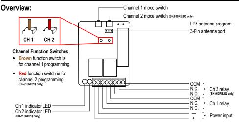
(PC board shown. Remove the front cover of the receiver to access the function switch(es) and terminal block.
