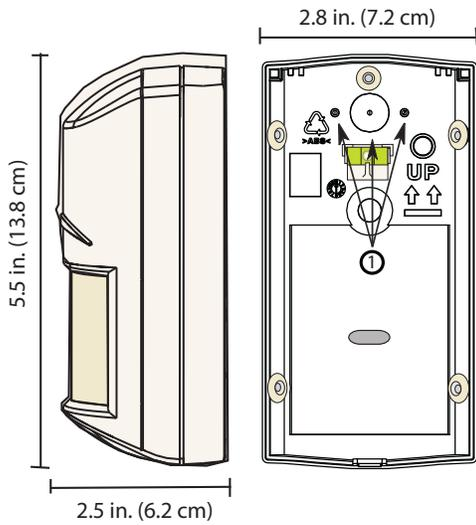
① Mounting holes. Punch out to receive screws.
