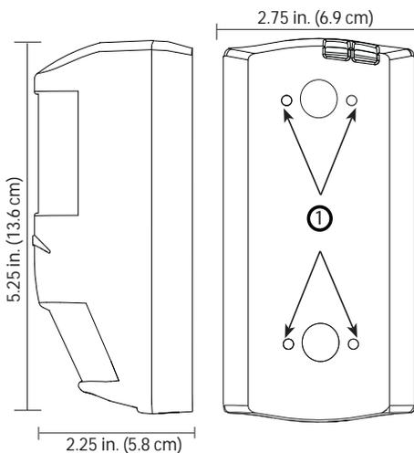
① Mounting holes. Choose one set and punch out to receive screws.
