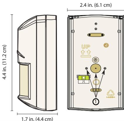
① Mounting holes. Punch out to receive screws.
