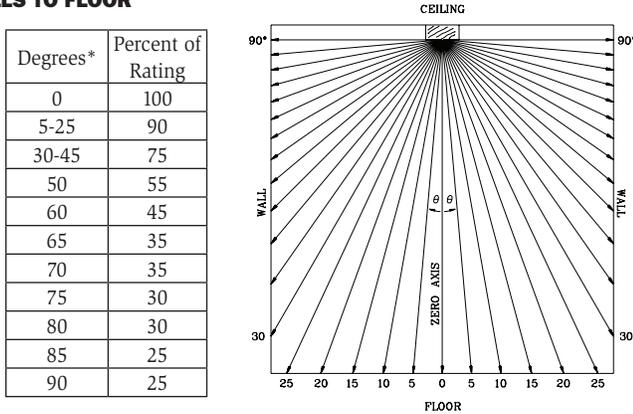
Figures 1-3 list the minimum light output requirements per UL1971.
