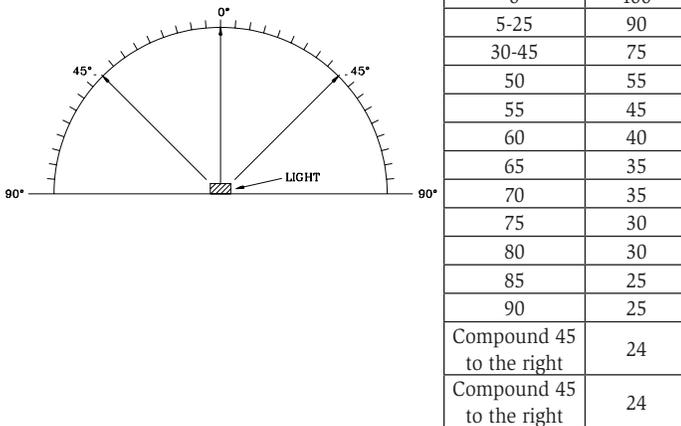
**FIGURE 3. LIGHT OUTPUT - VERTICAL DISPERSION, WALL TO FLOOR**
