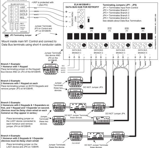
The above examples are intended to show the flexibility provided by the 4 data bus branches of an M1DBHR. The number and types of devices used on each branch is up to the Installer.
