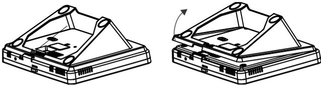
2. Remove the touch screen from the mounting base pressing the opening button on the bottom of the touch screen (as shown in Figure 2). In case the parts stick to each other, try to separate them by inserting a small screwdriver into the opening slot beneath the protruding opening button (Figure 2).
