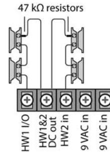
**Note:** Do not install the resistor at the panel terminals. This does not provide supervision of the wire.
