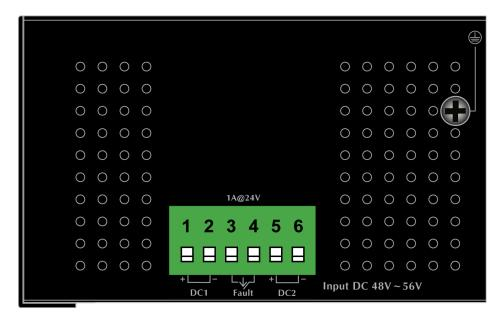
2. Tighten the wire-clamp screws to prevent the wires from loosening.
