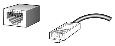
There are eight wires on a standard UTP/STP cable and each wire is color-coded. The following shows the pin allocation and the color of the straight cable and crossover cable connection:
