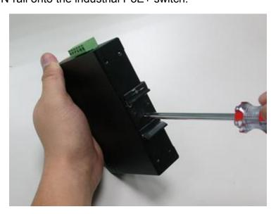
2. Carefully slide the DIN-rail into the track.
