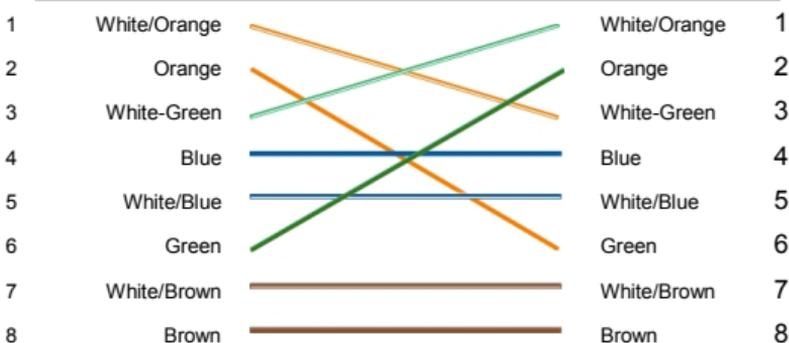
Ensure that the connected cables have the same pin assignment and color as above before deploying them in the network.
