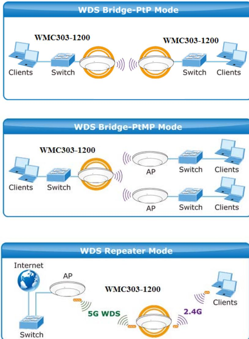
Before configuring the WDS Setting page, you have to select the wireless mode to “**WDS**” on the **WLAN2 (2.4GHz)** -> **Basic Settings** web page.
