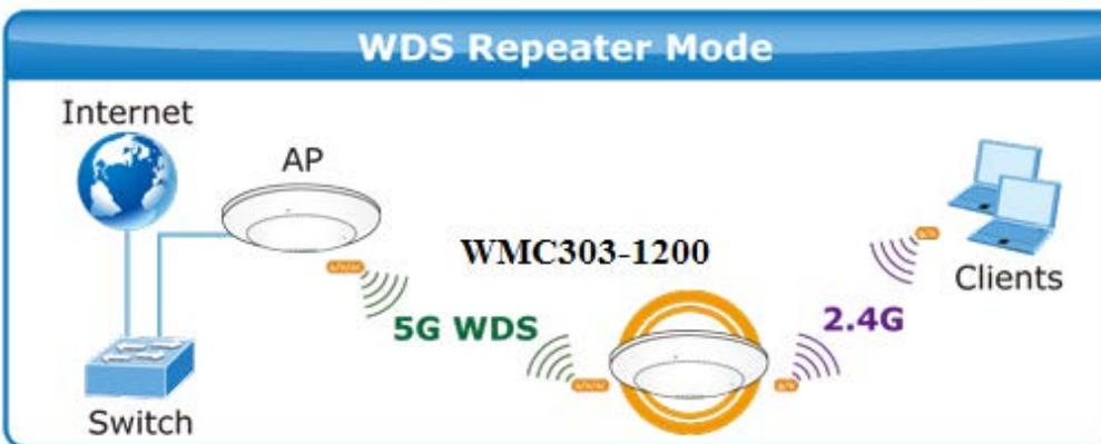
Before configuring the WDS Setting page, you have to select the wireless mode to "WDS" on the **WLAN1 (5GHz)** -> **Basic Settings** web page.
