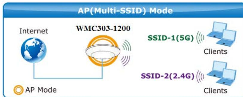
Choose menu “**WLAN1 (2.4GHz) → Basic Settings → Multiple AP**” to configure the device as a general wireless access point with multiple SSIDs.
