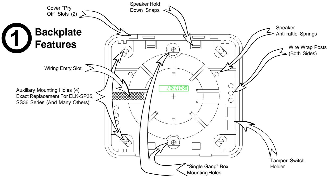
When replacing an existing ELK-SP35, SS36, or similar unit, the wiring condition shown below may be encountered
