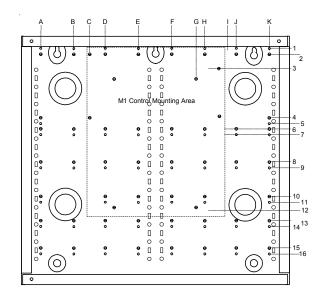
5. For accessory circuit boards there are 8 columns of repeated 2-hole punch patterns. These are labeled A, B, D, E, F, H, J, & K on the box diagram. One hole in each pattern is slightly larger than the other. These 2-hole patterns are for plastic Circuit Board Glides (p/n ELK-SWG). The small hole is for a 6/32 type "F" mounting screw and the large hole is for a half-moon shape Itab on the bottom of each glide.
