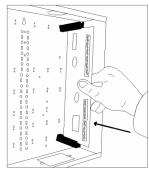
The circuit board should slide freely into the grooves between the two glides. If the board is loose or too tight, simply loosen one of the mounting screws and adjust the glide to assure a good fit.
