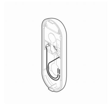
5. Crimp the two wires coming through the backplate to the existing wires threaded through the mounting bracket.
