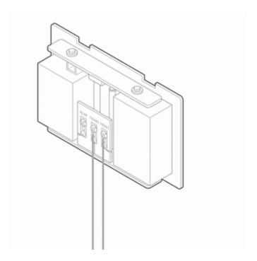
**Note**: The power module must be used in every installation regardless of the chime type. The power module is used to prevent the chime from buzzing or humming, and it helps ensure sufficient power is provided to the Alarm.com Video Doorbell.
