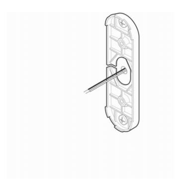
6. Install the doorbell backplate to the mounting bracket using the included machine screws.
