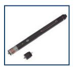
VFL (Visual Fault Locator): The visual fault locator can find breaks in fibers or high losses around connectors in simplex cables. The light that escapes at a break, for example, will be visible through the jacket of the cable.
