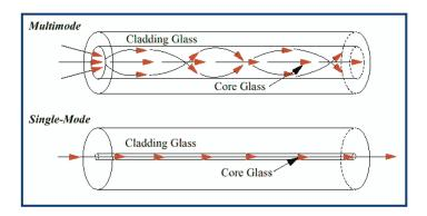
Multimode fiber has a relatively large light-carrying core, usually 50 microns or larger in diameter. It is usually used for short distance transmissions with LED or laser-based fiber optic equipment
