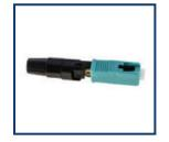
SC: A 2.5mm snap-in connector widely used in single mode systems for its excellent performance and in multimode systems because it was the first connector chosen as the standard for TIA-568. It is a snap-in connector that latches with a simple push-pull motion. It is also available in a duplex configuration.
