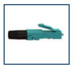
LC: A Lucent connector uses a 1.25mm ferrule, half the size of the ST and SC. Otherwise, it is a standard ceramic ferrule connector, favored for single mode. It is also the connector of choice for multimode transceivers gigabit speeds and above.
