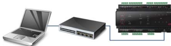
Ethernet 10/100 Switch hub Connection
