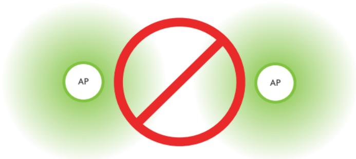
Ideally, roaming clients should see signal strength of two overlapping APs in the range of -60 to -70 dBm at the midway point between two APs
