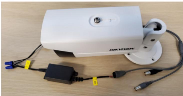
Figure 52, Dual Voltage Converter/Filter Installed
