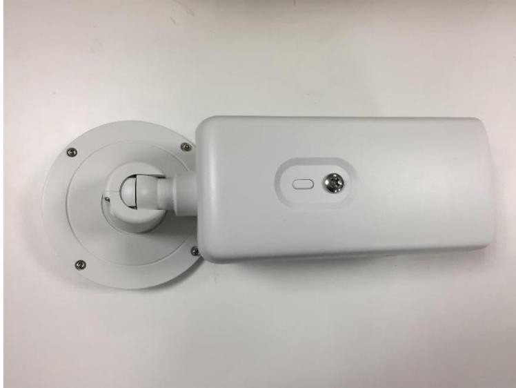
**Step4:** Unscrewing the screws to adjust the lens angle in order to adjust the image to the required monitoring site.
