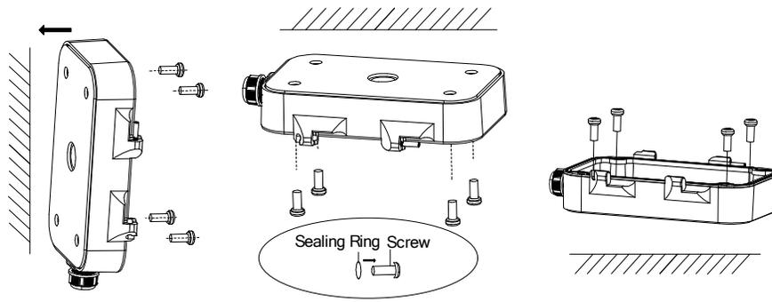
Figure 31, Install Junction Box Base
