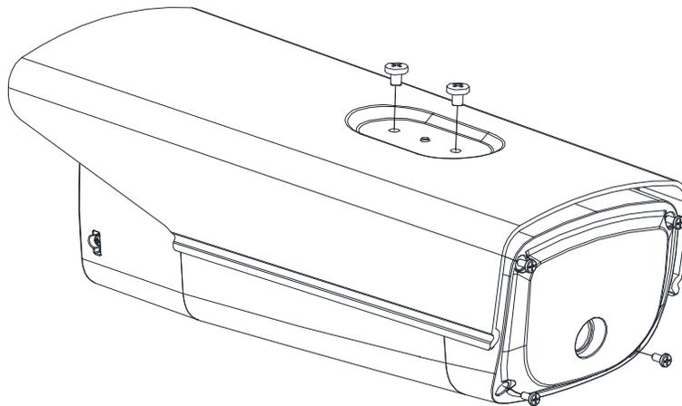
Figure 14, Figure 1-1 Fix Sun Shield and Back Cover
