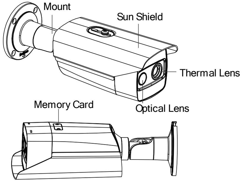
Figure 5, Type II Camera Appearance
