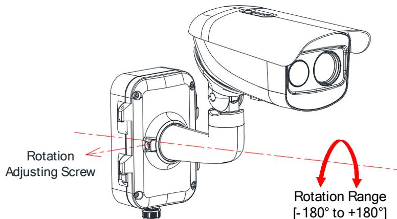
Figure 33, R-Axis Adjustment
