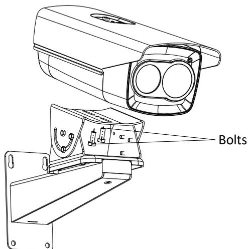
Figure 20, Fix the Camera to the Bracket
