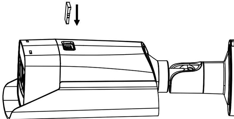
Figure 16, Insert MicroSD Card
