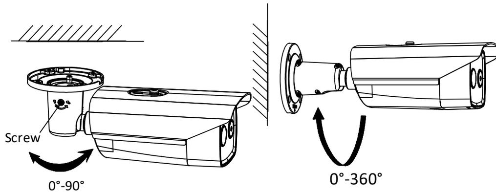
Figure 27, 2-Axis Adjustment
