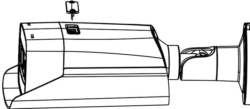
Figure 15, Remove Card Slot Cover
