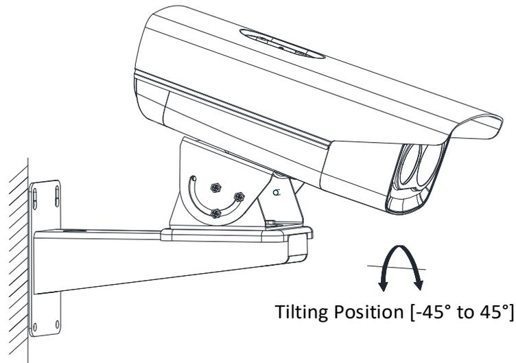
Figure 23, Tilt Adjustment
