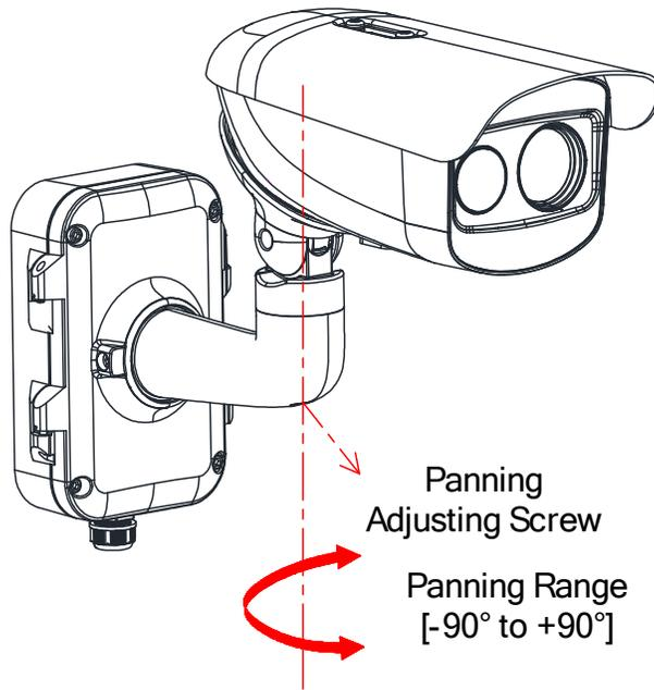
Figure 35, P-Axis Adjustment
