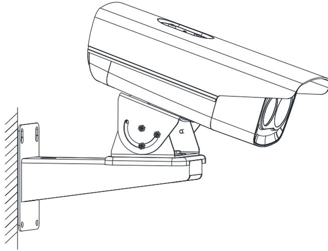
Figure 21, Fix the Camera to the Wall
