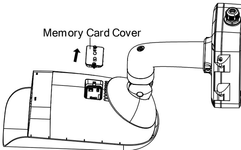
Figure 17, Remove Card Slot Cover
