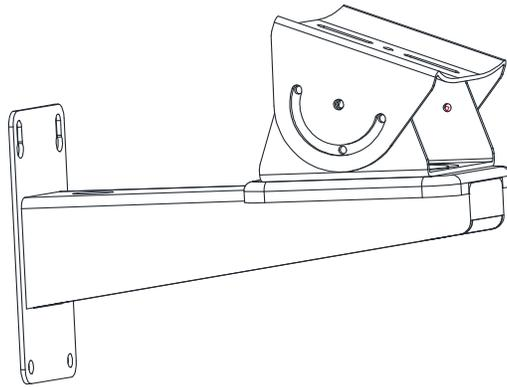
Figure 4, Wall Mounting Bracket (Optional)
