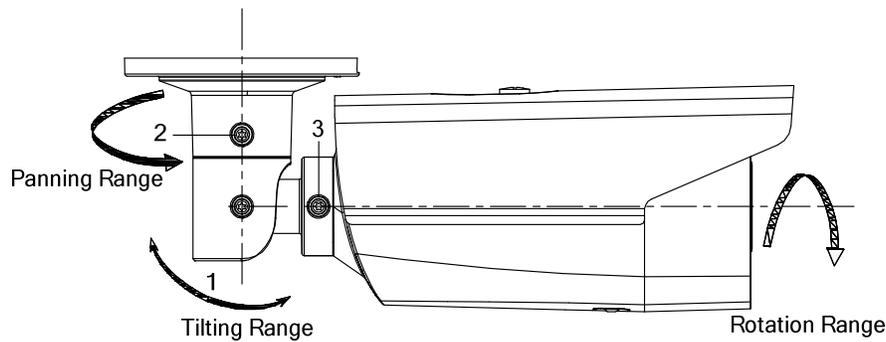
Figure 26, 3-Axis Adjustment
