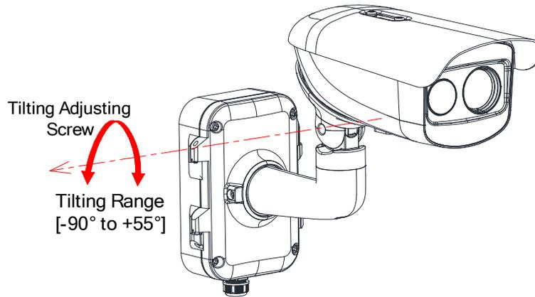
Figure 34, T-Axis Adjustment
