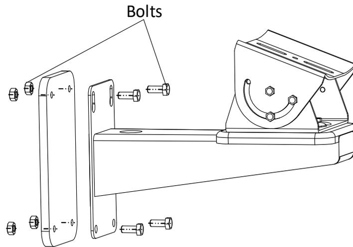
Figure 19, Install the Bracket onto the Wall
