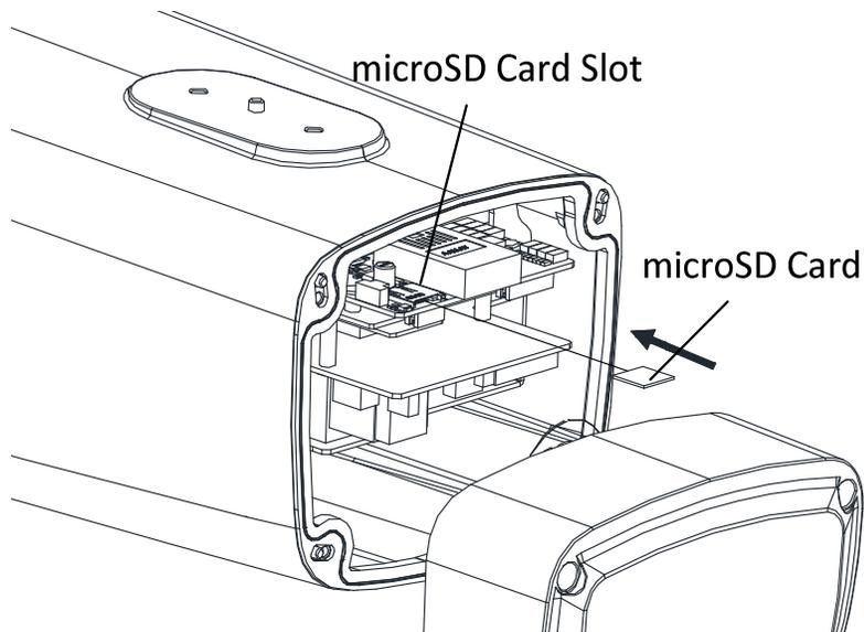
Figure 13, Insert MicroSD Card
