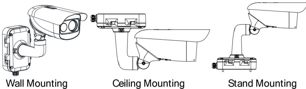
Figure 28, Type III Camera Installation Methods
