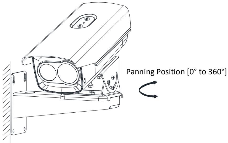
Figure 22, Pan Adjustment
