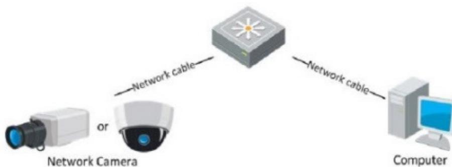
Figure 39, Connect via a Switch or a Router
