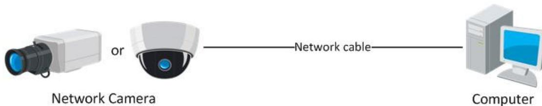
Figure 38, Connect Directly
