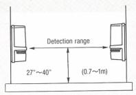
Maximum distances between Receiver and Transmitter are
