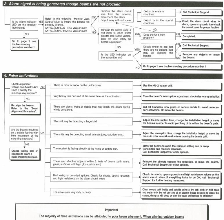
accept no less than an "EXCEL" value for the most stable and trouble free system !! Refer to the installation manual for acceptable Monitor Jack Voltage Values.
