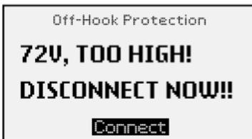
**Figure 4.2** Over Current Detection Warning
