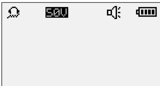
The MON position (MONITOR mode) causes the RECON Test Set™ to use its high impedance amplifier so that you can listen to a line without loading it. On-hook Caller ID is also received, checked and displayed in this mode. The line voltage is measured and displayed, with reverse polarity indicated by a reverse video icon. The RECON Test Set™ also monitors the line it is connected to for DTMF signals. If it detects any of the 16 valid DTMF signals it will display the characters on the LCD.
