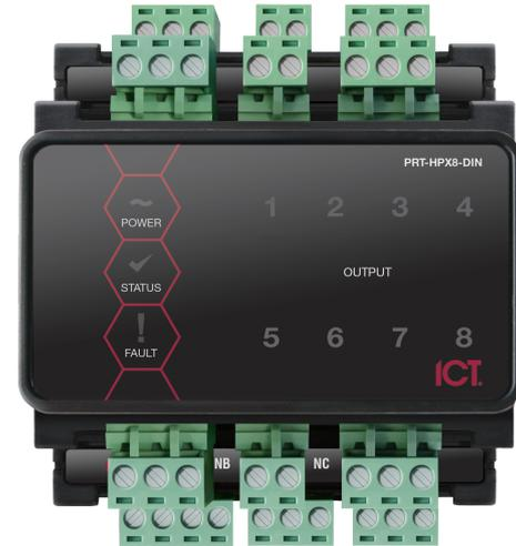
The Protege Half DIN Rail 8 Output Expander extends the Protege integrated access control, security and building automation system with an additional 8 outputs for automation.
