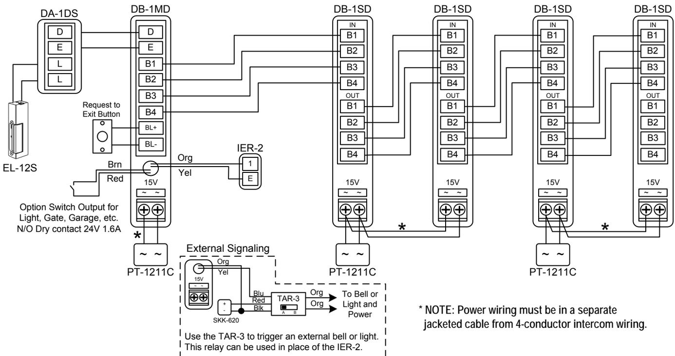
\* NOTE: Power wiring must be in a separate jacketed cable from 4-conductor intercom wiring.
