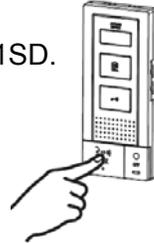
3. The LED will stop flashing to indicate that the ID registration is complete for that unit.
