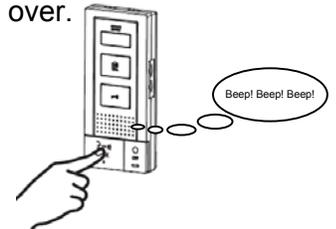
To reset an ID, push and hold the OFF button while pushing the TALK, CALL, and DOOR RELEASE buttons simultaneously.
