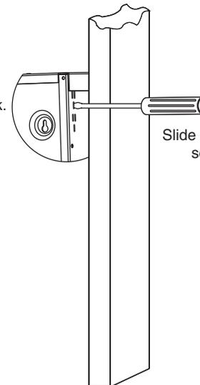
Slide enclosure on screw until screwdriver hits stud.
