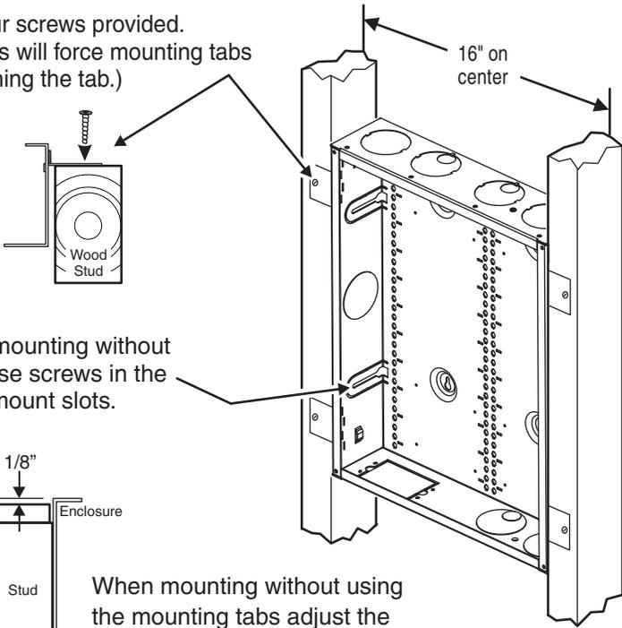
Or, when mounting without the tabs, use screws in the four side mount slots.
